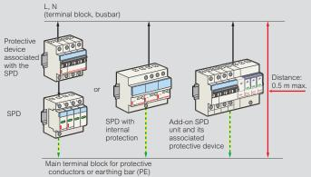
Connection lengths: as short as possible (< 50 cm if possible). EMC (Electromagnetic Compatibility) rules: avoid loops, fix the cables firmly against the exposed metal conductive parts of the enlcosure.
