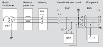
P1: main protection of the installation SPD: surge protective device with Uc 275 or 320 V recommended
